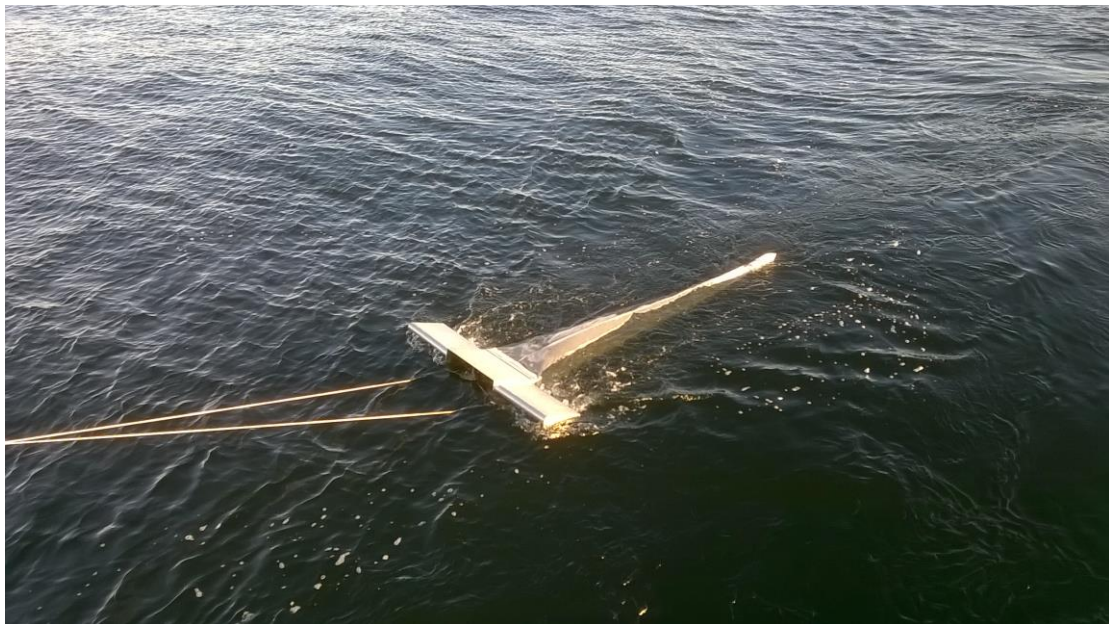
Figure 7. Launch of the Manta trawl used for monitoring microlitter particles in the surface water. Photo: Maiju Lehtiniemi.
