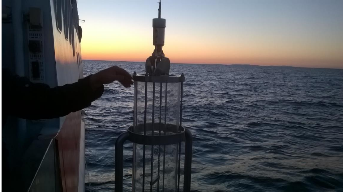
Figure 6. Launch of the water sampler used for monitoring phycotoxins from different water layers (between 0-10m). Photo: Maiju Lehtiniemi.
